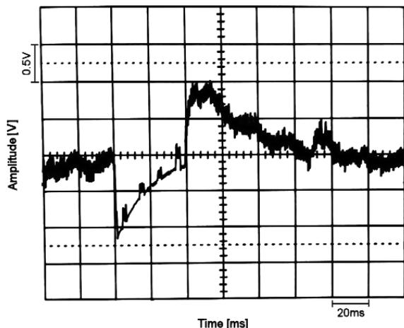
Fig. 3 - The waveform was captured from the screen of a digital scope. The signal was recorded on April 6, 2009 at 00:16 UTC and shows a negative pulse with an amplitude of ~1.2 Volt and a positive pulse with an amplitude of ~1 Volt and a frequency of ~10 Hz.
