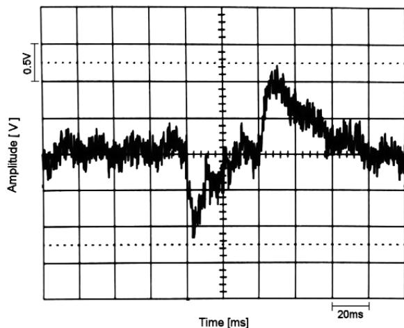
Fig. 2 - The waveform was captured from the screen of a digital scope. The signal was recorded on April 5, 2009 at 00:50 UTC and shows a negative and positive pulse with an amplitude of 1.2 Volt and a frequency of ~10 Hz.
