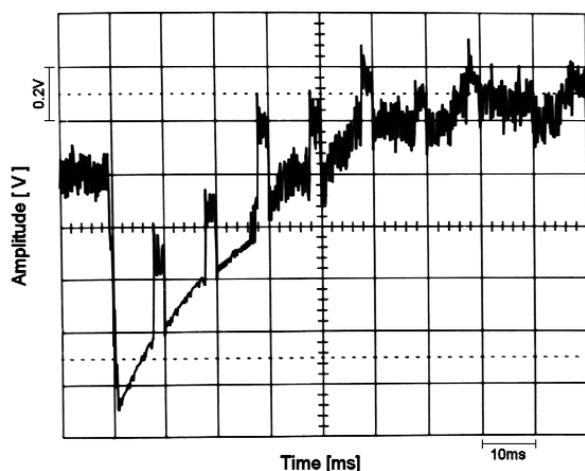
Fig. 1 - The waveform was captured from the screen of a digital scope. The signal was received on April 2, 2009 at 21:53 and shows an 880 mV main negative big pulse of 40 ms time width followed by a regular pulse sequence with a decreasing amplitude and a higher frequency of 100 Hz.
